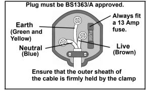
connected to the terminal which is marked E or  $\,\downarrow\,$  or coloured green.
